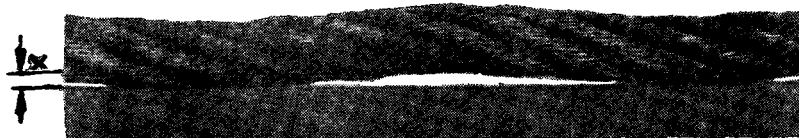
FIG. 12 WIRE ROPE WITH CORKSCREW DEFORMATION
