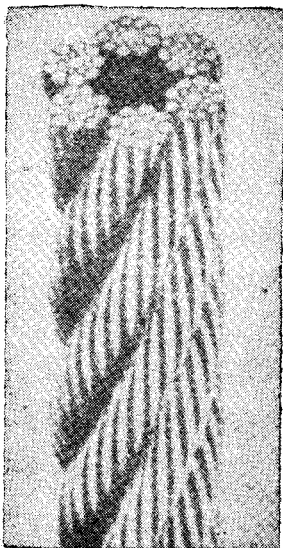
Ordinary Lay-Wires in Strand Spiral to Left
