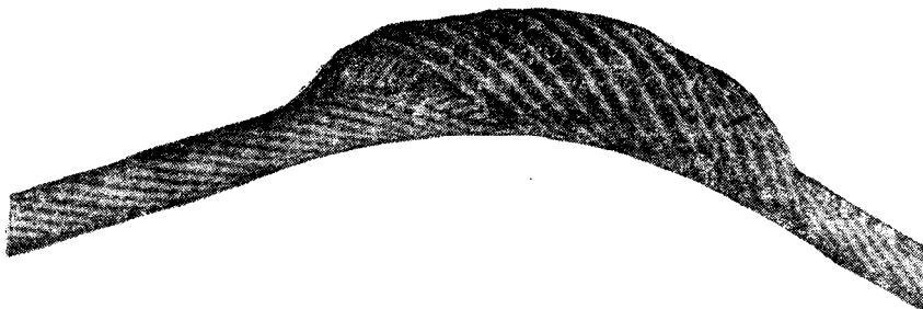
FIG. 13 WIRE ROPE WITH CAGE FORMATION
