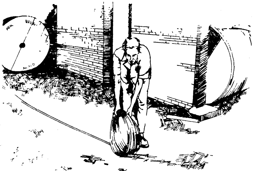
FIG. 5A CORRECT WAY OF UNCOILING
