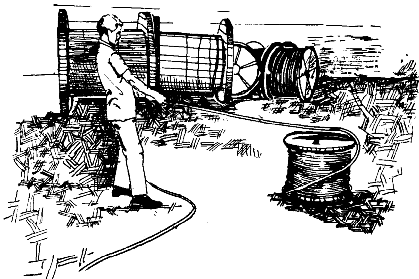
FIG. 4B INCORRECT WAY OF UNREELING
