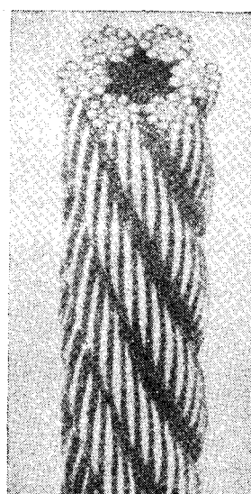
Ordinary Lay-Wires in Strand Spiral to Right
