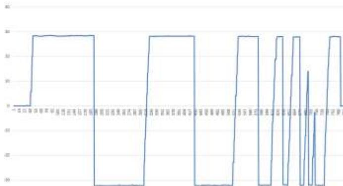
**The V2G fast charger was able to respond to change of charging current and change of power flow direction commands within 1-2 seconds after the commands are received by the charger.**
