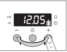
After approx. 5 seconds, the flashing stops and the clock displays the time of day set.
