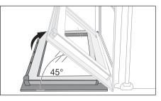
4. Take hold of the oven door with a hand on each side and pull it away from the oven at an upwards angle (**Take care:** It is heavy).
